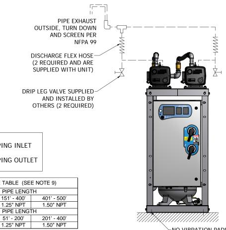
FIELD PIPING INLET ==== FIELD PIPING OUTLET EXHAUST PIPE SIZE TABLE (SEE NOTE 9) UNIT SIZE 151' - 400' 0' - 150' 1.00" NPT DPX 1.5 HP 1.25" NPT **UNIT SIZE** 0' - 50' 51' - 200' DPX 2 HP 1.00" NPT 1.25" NPT NO VIBRATION PADS ARE **NECESSARY AT THIS LOCATION** EFFECTIVE PIPE LENGTH TABLE FOR ELBOWS 1.0" NPT 1.25" NPT 1.5" NPT 2.0" NPT PIPE SIZE (IN)
