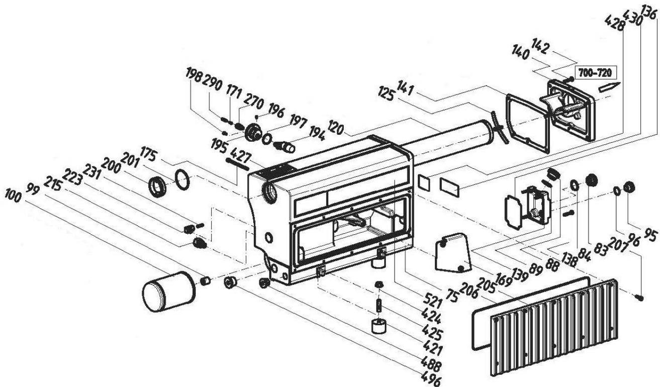
**Figure 6.3 Exhaust Filter (5 Hp RA0155)**
