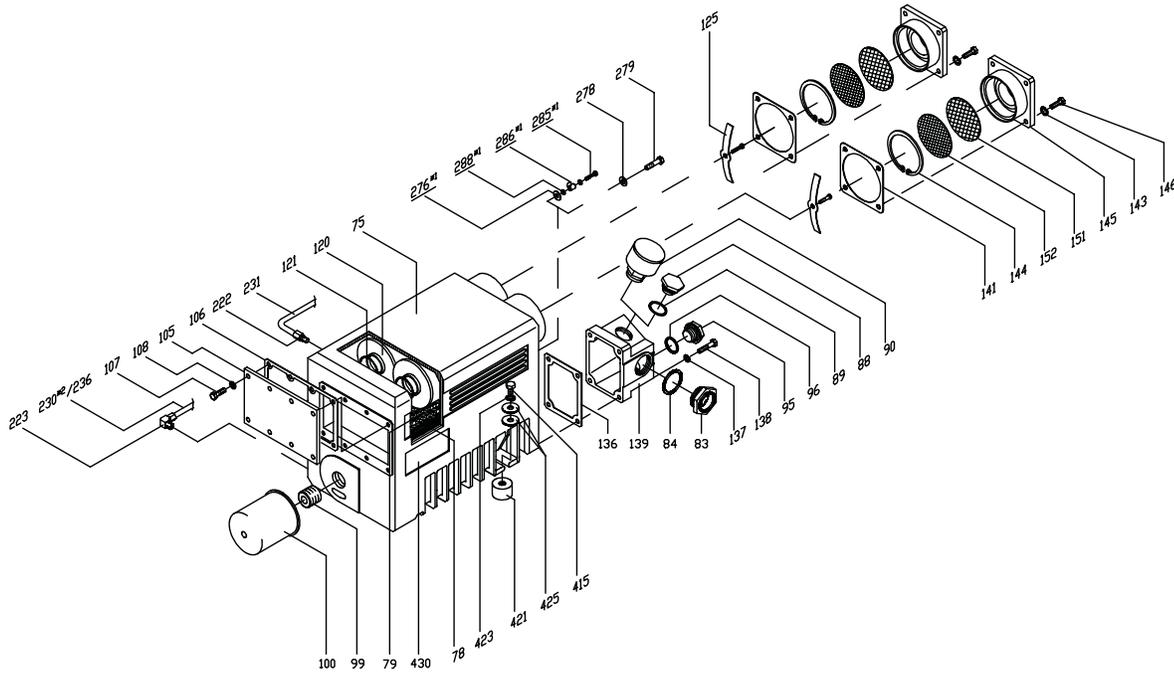
**Figure 6.2 Exhaust Filter (1.5 Hp through 5 Hp RC0101 and RA0100)**
