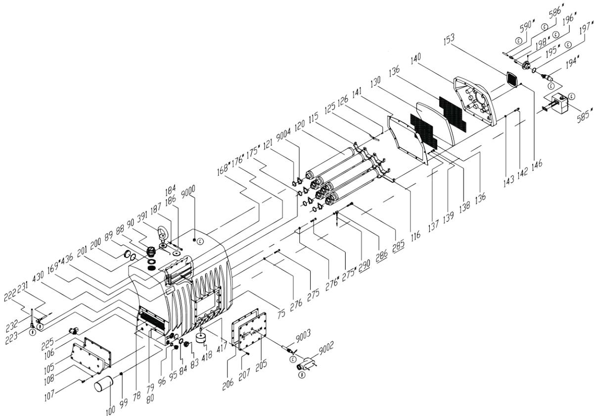
**Figure 6.5 Exhaust Filter (15 Hp through 25 Hp)**
