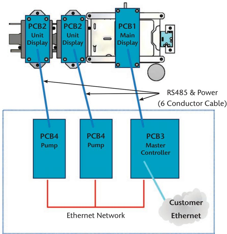
PCB3 & PCB4 Mounted on Back Panel
