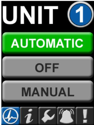
Figure 3A.5 Unit Screen - Automatic Mode
