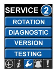
By observing the cooling fan of the motor, you can determine the rotation of the pump. After pressing the "Rotation" button on the touchscreen, there is a 5 second delay before the pump will start for a brief amount of time. Pump rotation should be counterclockwise when looking at the rear of the motor. Directional arrows are located on each pump.
