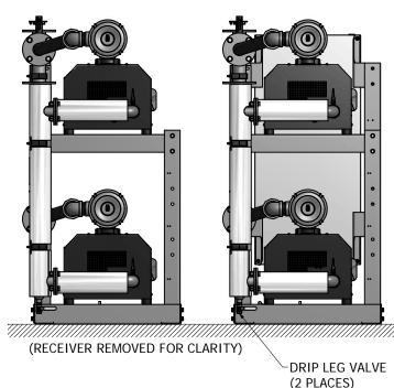
HOSPITAL-CONNECTION (4" FLANGE) EXHAUST PIPE SIZE TABLE (SEE NOTE 9) PIPE LENGTH UNIT SIZE 0-100' 101'-350' 351'-500' DISCHARGE-QX 10 4.00" NPT 5.00" NPT 6.00" NPT 3" FLANGE (2 PLACES) ······ 24 VDC ELECTRICAL – – FIELD PIPING INLET
