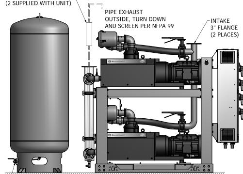
TANK DRAIN CONNECTION - CONTRACTOR SHALL PIPE
