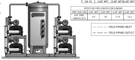
NO FOUNDATION OR INERTIA PAD IS REQUIRED (HOUSEKEEPING PAD IS OPTIONAL)
