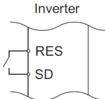
**NOTE:** OFF status of the start signal must be confirmed before resetting the inverter fault. Resetting an inverter fault with the start signal ON restarts the motor suddenly.
