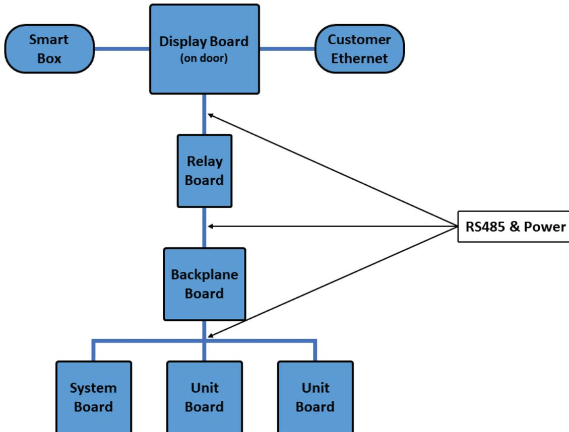
All Boards Other than Display Board Mounted on Back Panel
