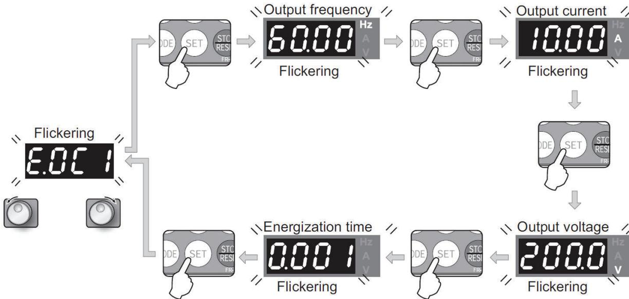
**Figure B1.3.2.1 Alarm Output Conditions (F700)**
