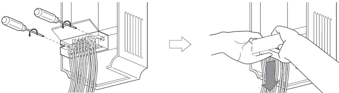
2. Using care not to bend the pins of the inverter's control circuit connector, reinstall the control circuit terminal block and fix it with the mounting screws.
