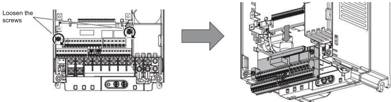
2. Using care to not bend the pins of the inverter's control circuit connector, reinstall the control circuit terminal block and fix it with the mounting screws.
