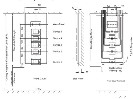
Semi-flush Fitting Up to five gases
