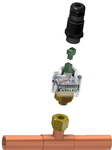
Figure 4: Remote Sensor Assembly Installation
