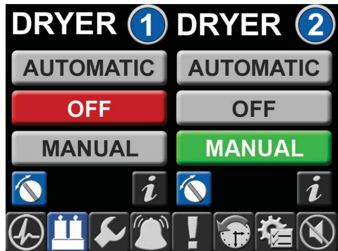
Figure 3.7 Main Screen - Dryer Operation
