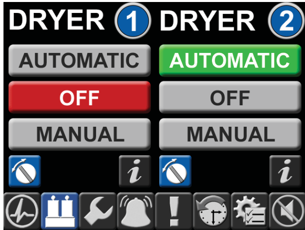
Figure A.1 Main Screen - Dryer Operation
